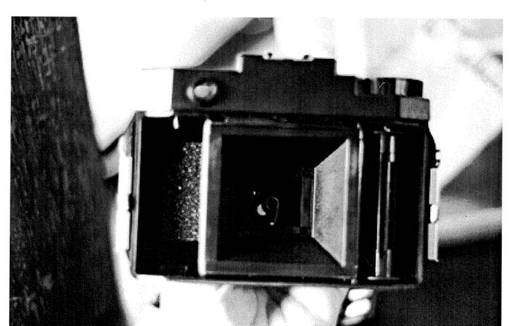
3. Remove the guide and notice the two small screws holding the lens on.
