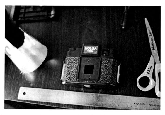
9. Measure the lens cavity, and transfer it to the can.
