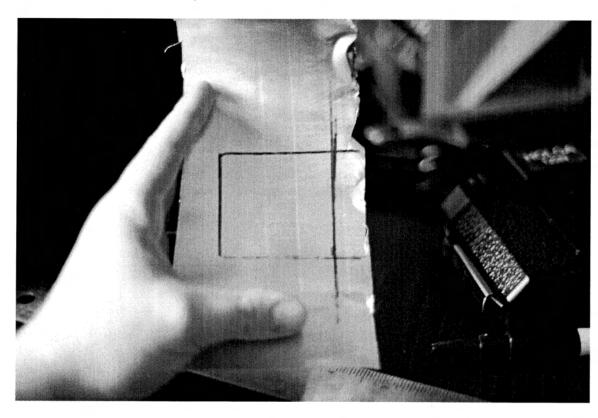
10. Do some trimming, measure the center, and fit the new aperture in place. Pierce the center with a needle, the smaller the better!
